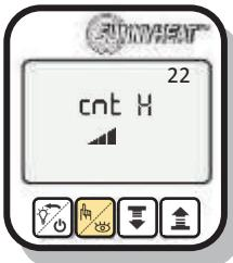
Press the 2nd button in the view level as often as the value is shown with the operating hours counter symbol.
