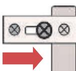
Turn the lock tabs into the open position, mount the heating panel and push in the direction of the arrows to the stop.
