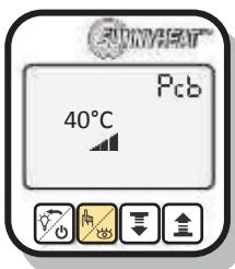
Press the 2nd button in the view level as often as the value is shown with the Pcb symbol.
