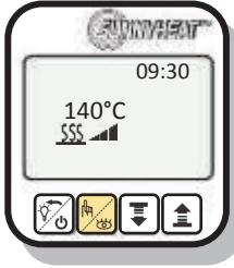
Press the 2nd button in the view level as often as the value is shown with the radiation temperature symbol.
