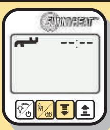
By simultaneously pressing the 2nd and 3rd button, you move from the main level to the view level. Press the 2nd and 3rd button again on the view level at the same time to enter the settings level.
