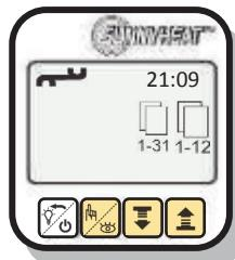
You can see the calendar day and the month. The calendar day is flashing, you can change this with the arrow keys. Then press the 2nd button, the month is flashing, you can also change this using the arrow keys.
