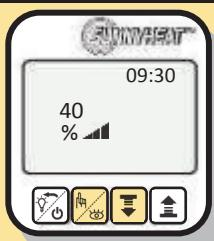
By simultaneously pressing the 2nd and 3rd button, you move from the main level to the view level.
