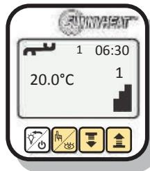
You will see different values of a heating program. Right above the heating program symbol, you will see the heating program number, this flashes. You are currently in the heating program 1, using the arrow keys move to a different heating program.
