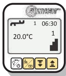
In the centre top edge, you will see the temperature profile number, it flashes. You are currently in the temperature profile 1 of the heating program 1.
