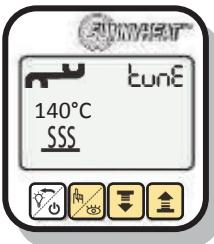
Press the 2nd button in the tune menu as often as the value is shown with the radiation temperature symbol.
