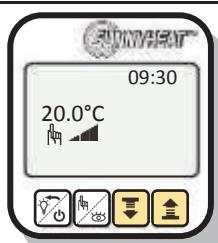
The desired temperature is the temperature to which your SUNNYHEAT heating panel should heat up. It is located above the hand symbol.
